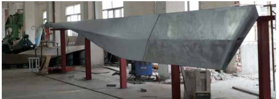
Factory mock-up for architectural fins
