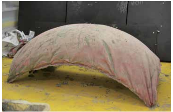
Experiment 1: Concrete shell stands on 4 points.
