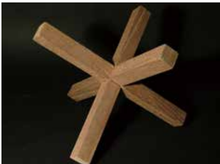
Experiment 6: Chidori Joint - How to make a secret timber joint? By Allison Choi Hau Ying, Min Fan Ka Man & Horace Yeung Chi Ho
