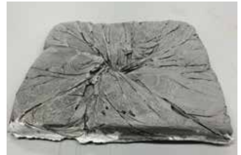
Experiment 2: First test model casted directly in a plastic bag.
