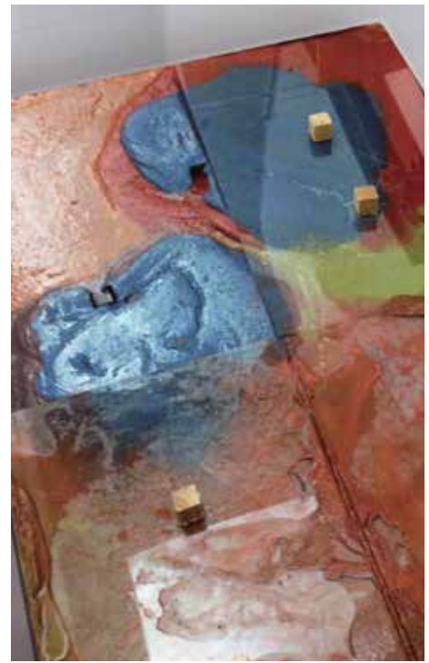
Experiment 3: Colourful patterns indicate sequences of concrete pouring.
