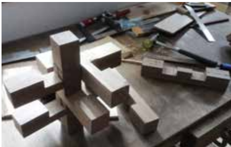
Experiment 5: Lu Ban Lock - How to make a secret timber joint? By Chloe Leung Shun Kiu & Kary Yuen Chun Yi
