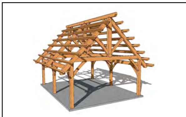
Figure A1.3a: traditional post and beam barn structure
