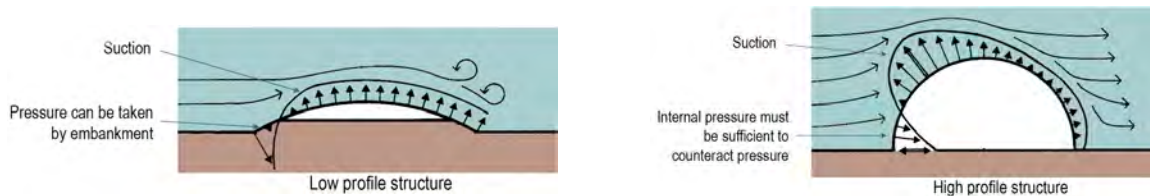
Figure E4.4: Wind Effects on Pneumatic Structures
