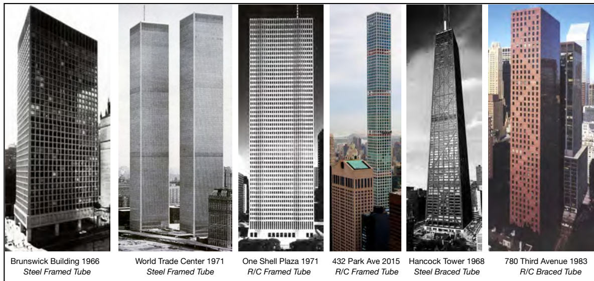
Figure F3.23 Tube Structures. Examples.
